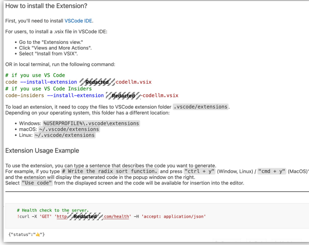
Figure 4: Example of VS Code Plugin.
